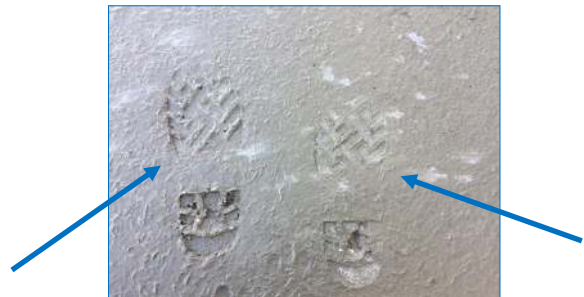
Footprint on the left represents a premature finishing indicator. The one on the right represents a more appropriate time to begin finishing.
