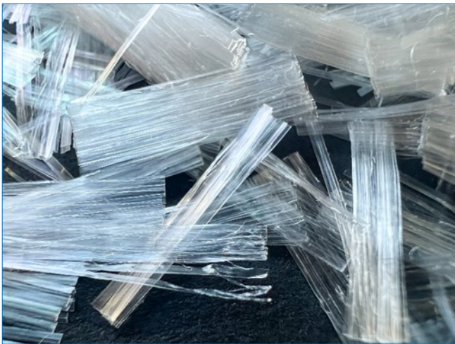
Typical fibrillated microfibers used for plastic shrinkage crack control are 0.75 inches in length and used at dosage rates of 1.5 to 3.0 lbs./cu.yd.
