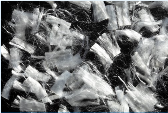
Typical monofilament microfibers used for plastic shrinkage crack control are 0.75 inches in length and used at the dosage rates of 0.5 to 1.0 lbs./cu. yd.
