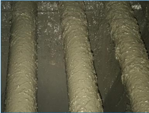
Rounded pump hopper grates significantly reduce the amount of FRC build up
