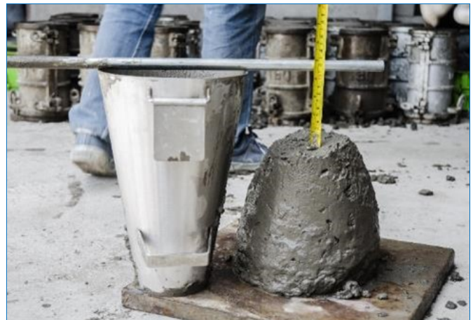
Slump loss can be expected when adding fibers to a concrete mix
