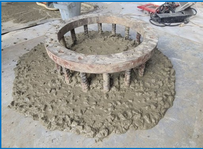
Figure 3. J-Ring test ent VSI for SCC mixes. Commonly used static segregation tests include Column Segregation [13]
