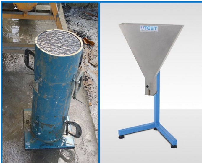
Figure 5. Column Segregations (left) and V-Funnel (right) Test Apparatus
