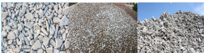
Figure B- Material life phases of concrete: recycled concrete, recycled concrete base, and landfill concrete.
